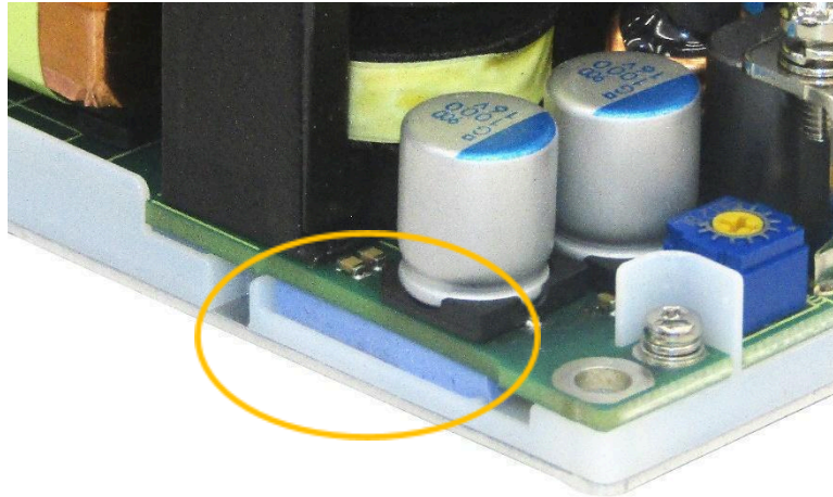
Figure 6: Gap filler between the printed circuit board and chassis
