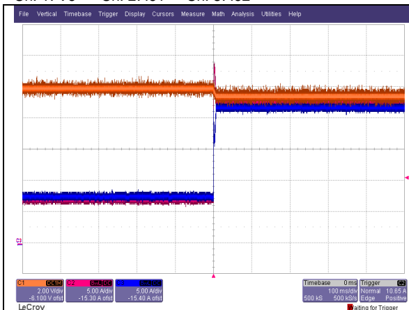
Load Transient Response. Load Step: 15A to 45A, 0.1A/us slew rate. Ch. 1: Vo Ch. 2: Io1 Ch. 3: Io2
