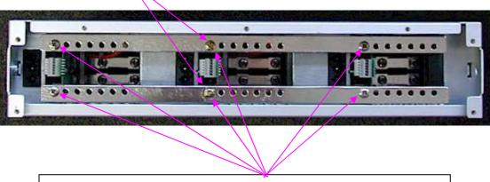
For Multiple load leads distributed load leads evenly as possible on all M5 Screws
