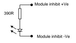
Internal to the module inhibit is a 3900hm 1/8W resistor and the diode of an opto-coupler.
