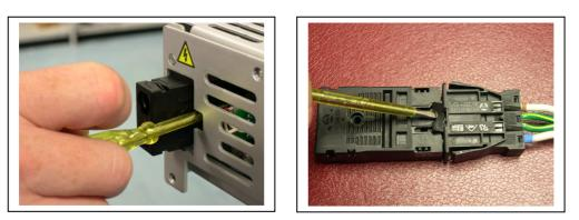
Insert a flathead screwdriver down the side of the connector as shown in photo, release the locking mechanism shown in the photo showing the locking tab and pull from the back of the unit (connector removed from the back of unit for purpose of illustration).
