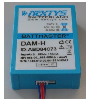
Figure 24: Cable connection to the DAM
