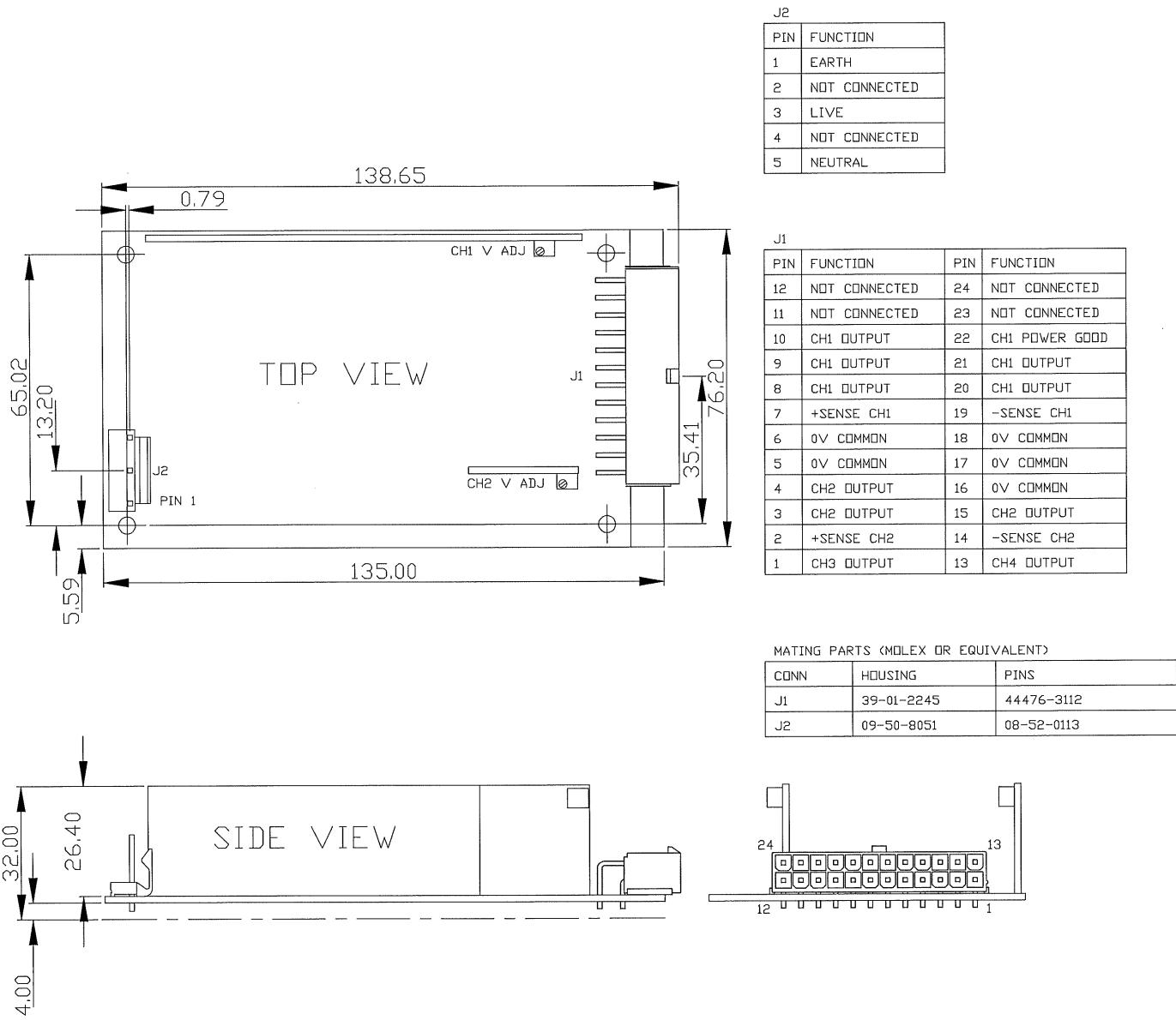
Note: The NVA1-E5K0 series J1 output connector pins 1 and 13 are channel 3 output.
