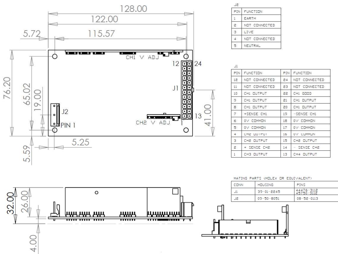
Note: The NVA1-E5K0 series J1 output connector pins 1 and 13 are channel 3 output.
